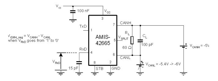
Figure 3. Differential Receiver High Threshold Voltage for CMV = -5 V
