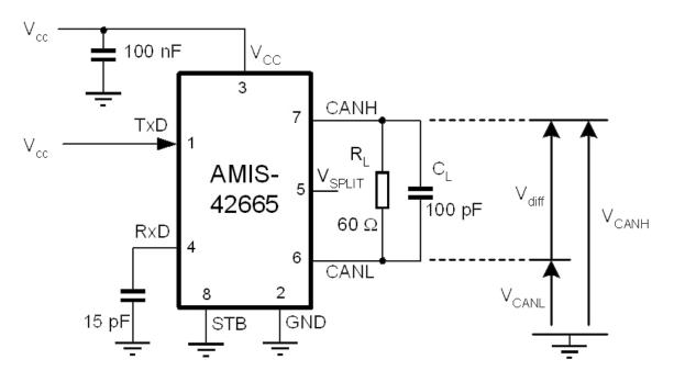
Figure 1. Set-up V<sub>CANH</sub> and V<sub>CANL</sub>
